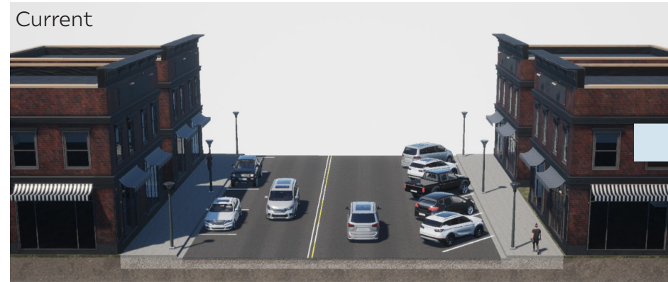
Very large space for cars (60'), limited sidewalk space (10' each side)
