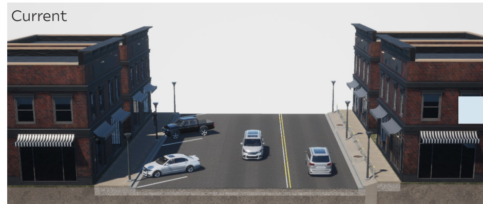
Very large space for cars (56'), limited sidewalk space (12' each side)
