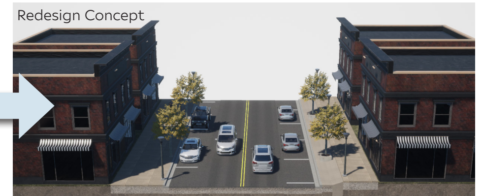
Parallel parking on both sides, allowing 16' to be reallocated to sidewalks
