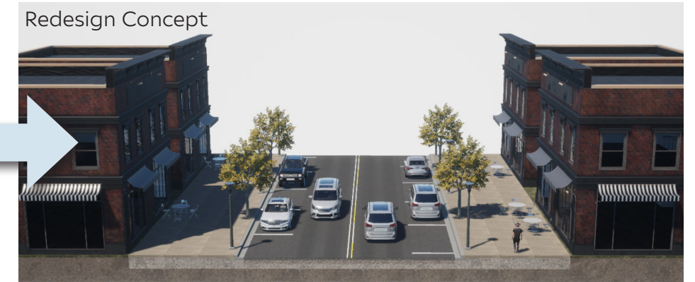
Parallel parking on both sides, allowing 30' to be reallocated to sidewalks
